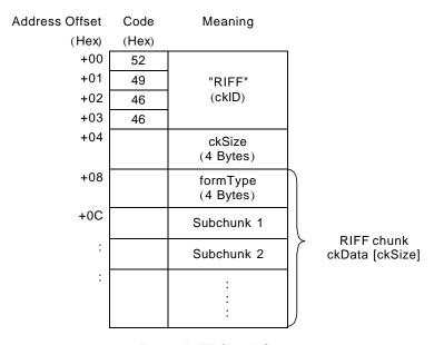
Fig. 31 RIFF Chunk Structure
