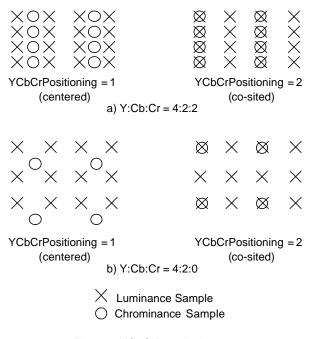
Fig. 8 YCbCrPositioning
