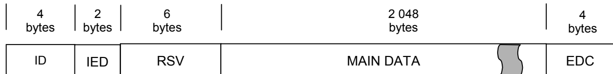
Figure 28 – Logical Layout of a DVD Data Sector
