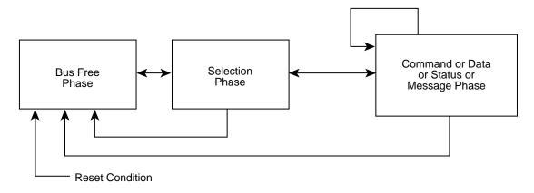
Figure 5. Phase sequences without arbitration
