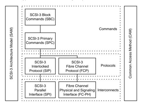
Figure 1. Functional scope of SCSI-3 standards
