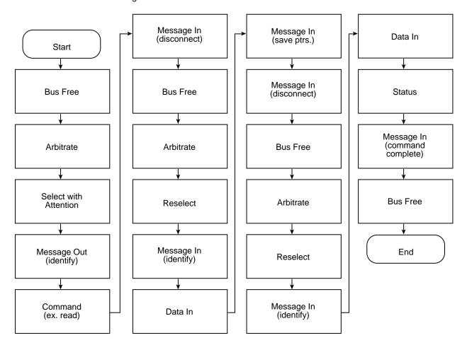
Figure 9. Disconnect example
