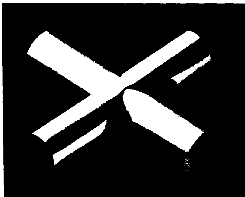
FIGURE 1.5: The concave edge of the union of two cylinders is blended with a constant radius fillet. The result cannot be modelled with standard surfaces.
