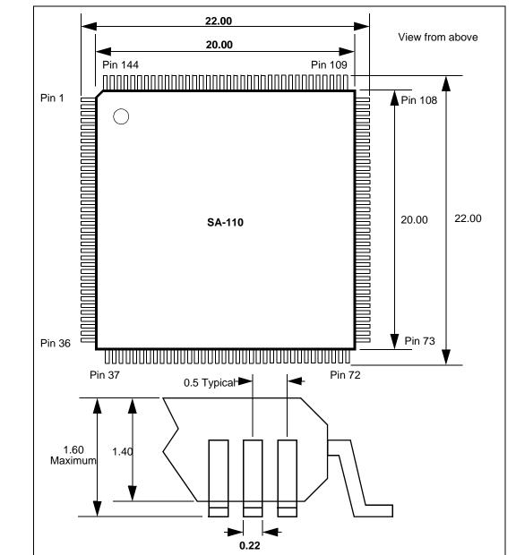
Figure 13-1. SA-110 144-Pin TQFP Mechanical Dimensions
