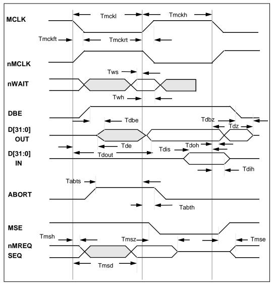
Figure 12-2. SA-110 Address Timing with APE=Low
