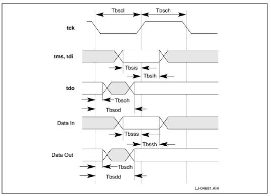
Figure 10-4. Boundary-Scan Tristate Timing
