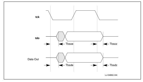
Figure 10-5. Boundary-Scan Reset Timing
