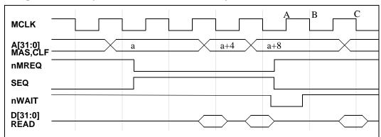
The SA-110 samples the **nWAIT** signal pin at time A. The signal **nWAIT** must meet setup and hold requirements with respect to the rising edge of **MCLK** at A. Without the stall cycle, the data would have been sampled at time B. Inserting a single stall cycle causes the data to be sampled at time C.
