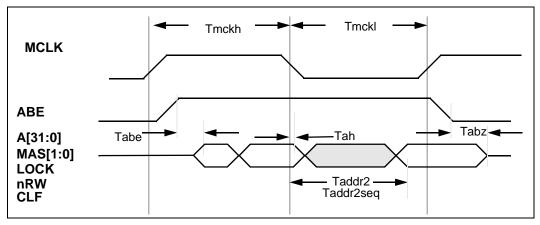
Figure 12-3. SA-110 Address Timing with APE=High
